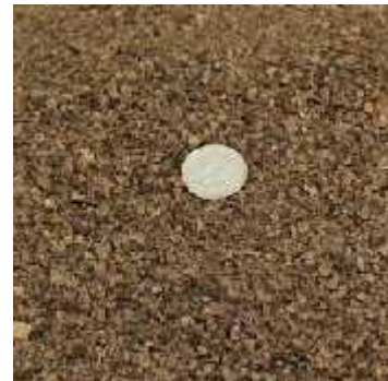
Fractured Gravel Screening – not smoothly round approx. size 2-5mm
