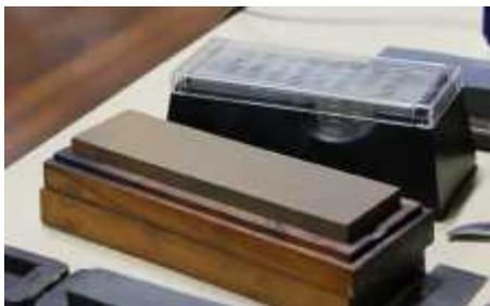
Basic sharpening tools are the diamond lap (above) and sharpening stone (below)
