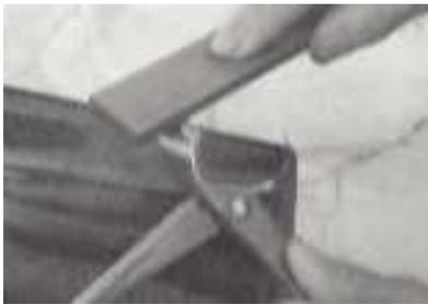
Step 2. The blade that crosses over the other is called the upper blade, and the one underneath is called the under blade. (The branch cutter is turned over in the picture, so that the blade you see on the top is the under blade.) The outside of the under blade is sharpened first. The blade is narrow at the tip; apply the whetstone flat against this part of the blade. As with shears, just a few light strokes are enough. Next carefully shave off the burr on the inside of the blade.
