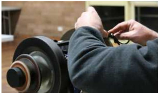
Professionals like John generally use an electric water wheel. The stone wheel spins constantly moistened through a tray of water during the sharpening process. Once the basic sharpening is done, the leather wheel on the opposite side is used for finishing and polishing.
