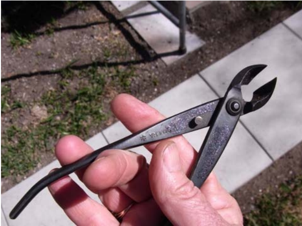
This is the correct way to hold side-cutters
